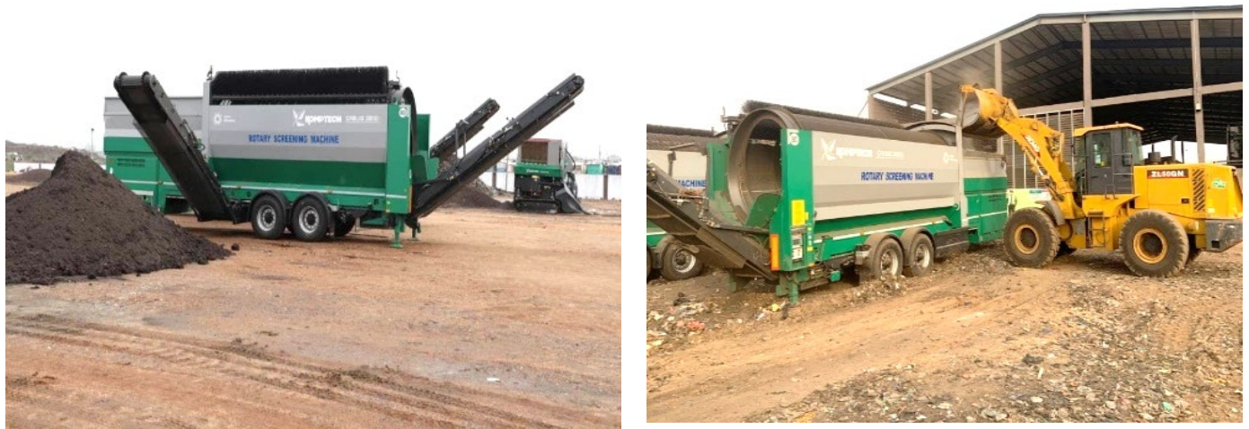
Figure 3.5 Typical Cribus 3800 Komptec and Wheel Loader
