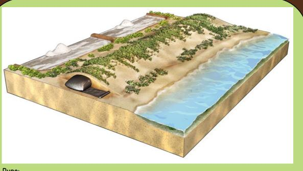
Option 3: Using geotextile tubes as dune construction
